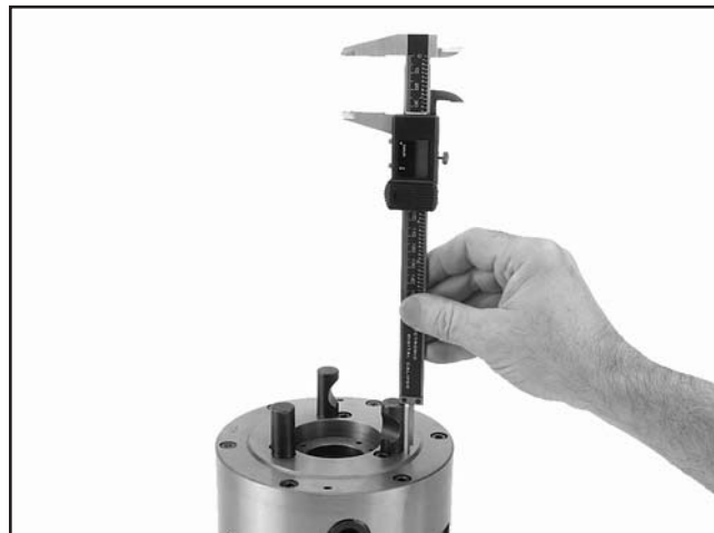
Figure 23. Measuring height of cam-lock studs.
